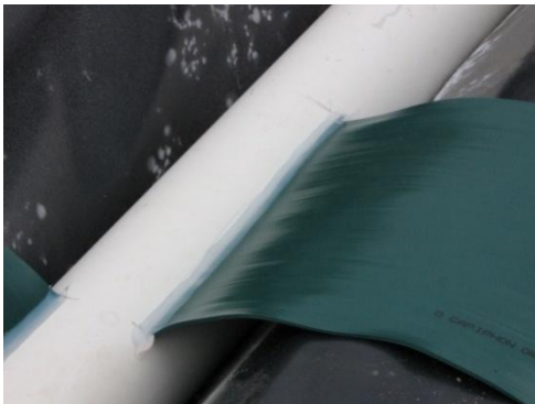
Figure 2. The Capiphon belt is usually inserted into a collection pipe laid some 10 cm below the level of the belt to increase the capillary head.
