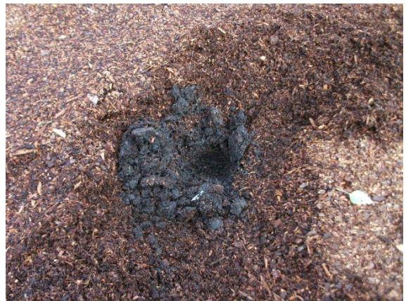
Figure 13b. A deeper hole under the swings in the drained area shows no sign of free water.
