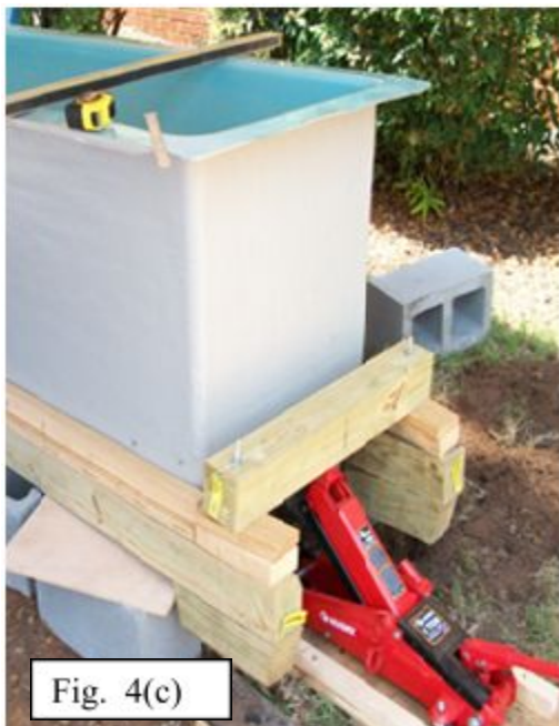
Figure4. Capiphon™ installations procedures in a fiberglass trough 3m long and 0.6 x 0.6m in cross section.
